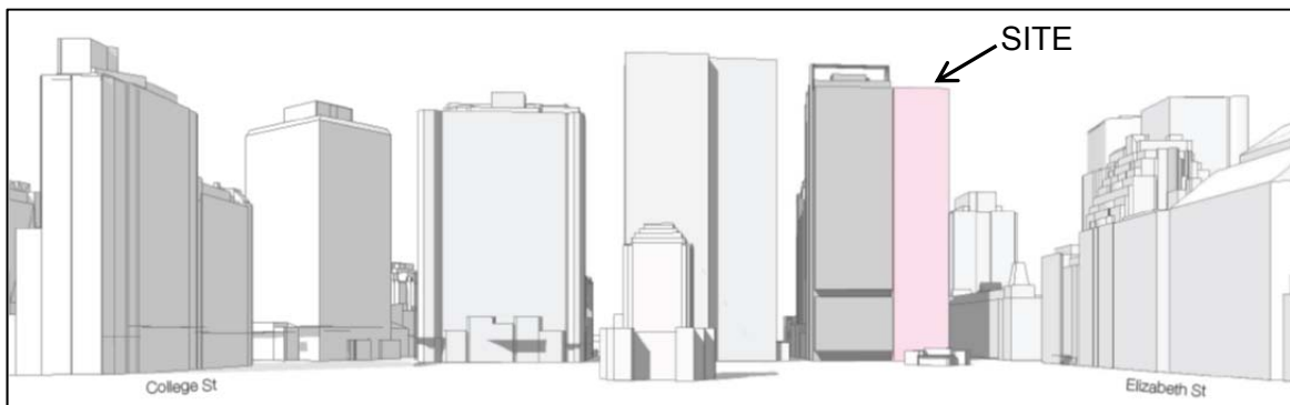
Figure 13: The approved Stage 1 DA building envelope massing as viewed from Hyde Park South, illustrating an envelope to a height of 110 metres
